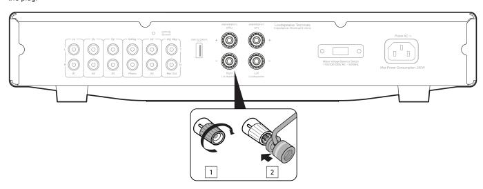
Connect the wires from your left channel loudspeaker to the Left positive and negative terminals and the wires from the right channel loudspeaker to the Right positive and negative terminals.
