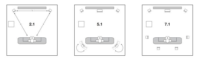
When using the MIN22 speakers with for TV and film, we recommend positioning the speakers above or below the screen, angled towards the listener where possible.
