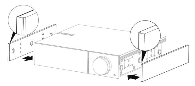
When installing new magnetic side panels, please ensure that the groove cuts are aligned with the direction of the front panel. Insert from the rear by holding the rear of the panel.
