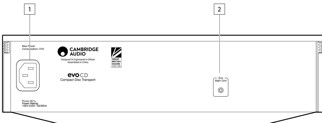
1. **AC Power socket** - Once you have completed all connections to the EVO CD, plug the supplied AC power cable into an appropriate mains socket then switch on. Your EVO CD is now ready for use.
