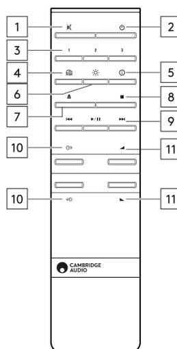
If the remote control will not function, please check that the batteries have not expired, and that there is nothing blocking the front panel IR sensor, which is located in the EVO 75/150. There is no IR sensor located in the EVO CD.
