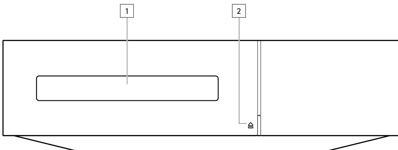
1. **Disc tray** - Used for the loading of compact discs, operated by the Open/Close button.
