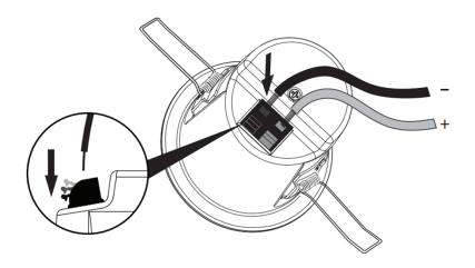
4. Next, press the metal clips upwards and fit the two longer arms into the ceiling hole.
