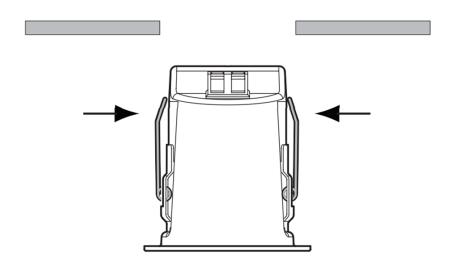
5. Push the speaker upwards until firmly within the mounting hole.
